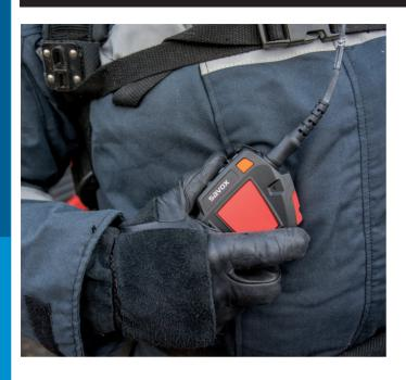
The SAVOX® C-C550 is a combined Remote Speaker Microphone and body worn Push To Talk unit. It is rugged and has been extensively tested (MIL-STD-810G) to provide robust and reliable communications for professionals working in harsh conditions. The C-C550 is dust proof and submersible in water to 1m (IP67).
